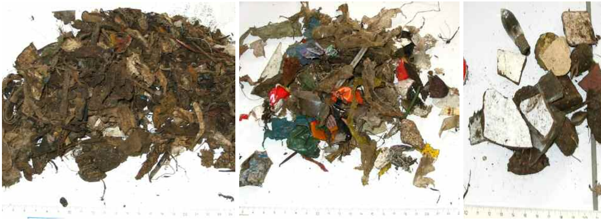
Figure 6 Material groups from intermediate fraction after manual sorting (input material: unshredded solid waste).
