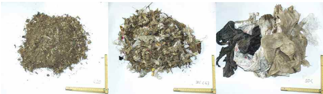
Figure 4 Sieve fractions (fine, intermediate, coarse) after dynamic treatment (input material: unshredded solid waste)
