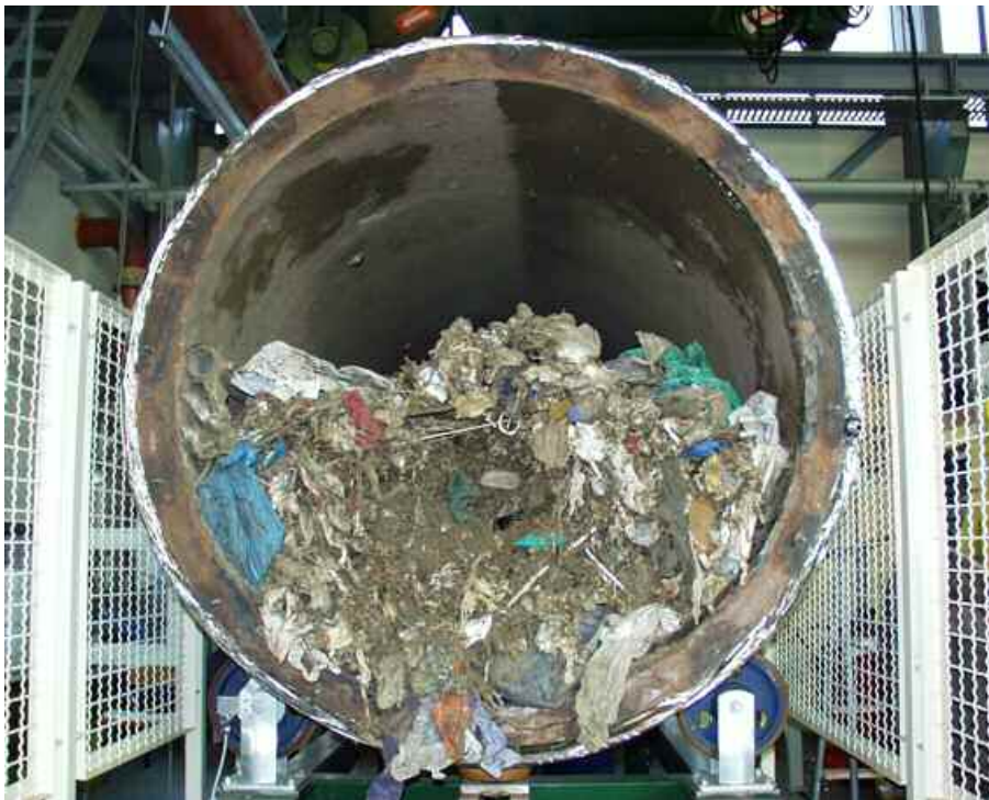
Figure 3 Open reactor at end of test (input material: unshredded solid waste)
